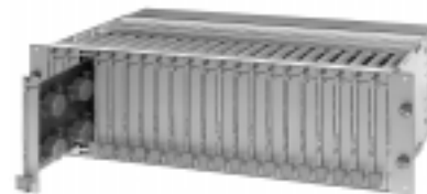
BT 901 with 21 plug-in modules
